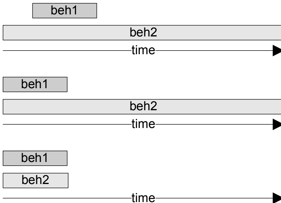
Figure 6.6: In all figures, behaviors beh1 and beh2 are two mutually exclusive behaviors. Top: beh1 and beh2 overlap during some interval of time. Since beh1 has the latest start time, it will be selected to play during the overlapping time interval. Middle: beh1 and beh2 share the same start time. Since beh1 has the earliest end time, it will be selected during the time interval on which the behaviors overlap. Bottom: beh1 and beh2 share the same start and end time, one of them is dropped and the SAIBA Behavior Planner is informed of this.
